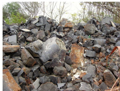
(d) Heap of slags, showing leftovers from the smelting process. (Pignata, 2006)
